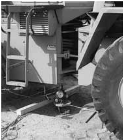
Figure 2 Plate Bearing Test
