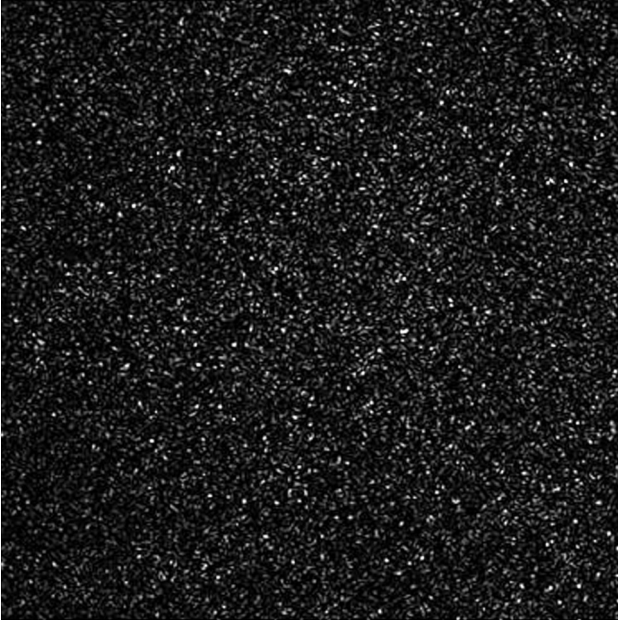
Figure 8 Speckle pattern generated by placing only a circular aperture instead of the filters.
